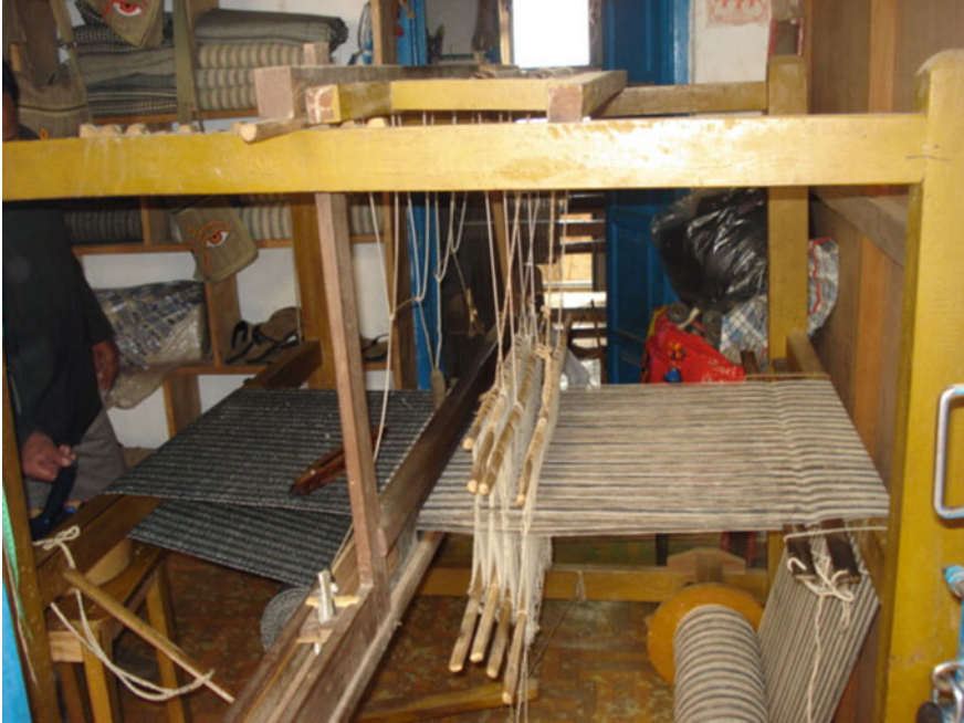
Fig. 23.8 Improved handloom to weave allo wool fabric
