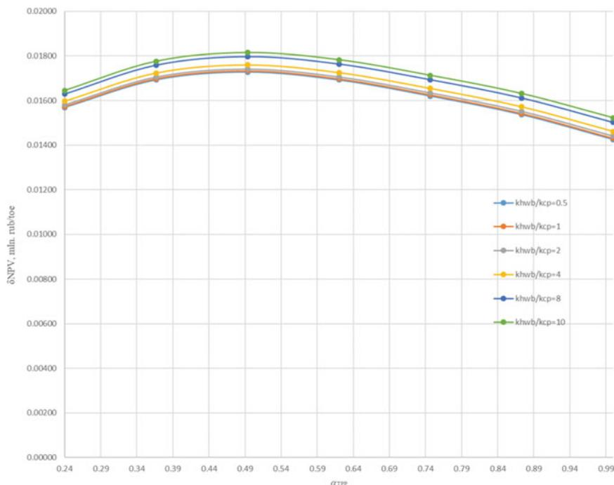
**Fig. 5** Increase of specific integral economic effect  $\delta NPV$  for different values of the extraction factor at different ratio of the specific cost of hot water boilers and steam heat exchangers
