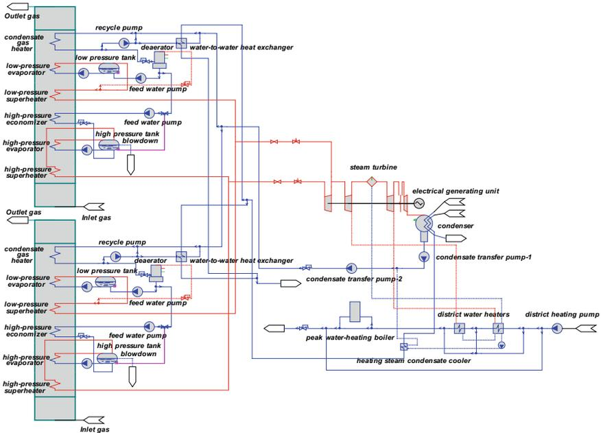
**Fig. 1** Basic diagram of a double-loop combined-cycle CCCP, simulated in the CAD “United Cycle”
