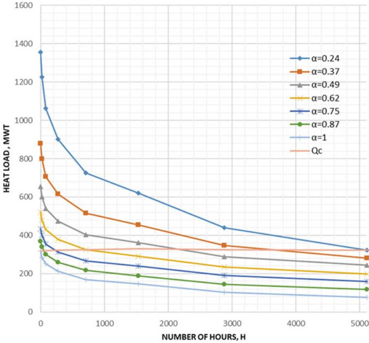
**Fig. 3** Dependence of the plant total heat load on the number of hours of outside air temperatures during the year for the heating period of St. Petersburg (Rossander's diagram)
