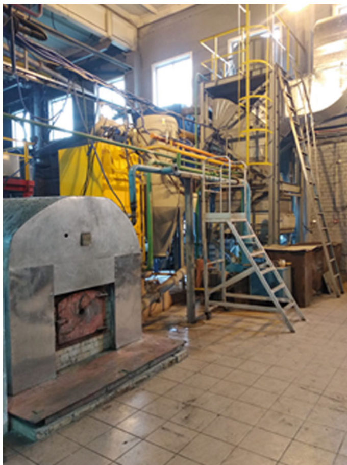
Fig. 3 The CWSF combustion block of experimental installation, Siberian State Industrial University, Russia
