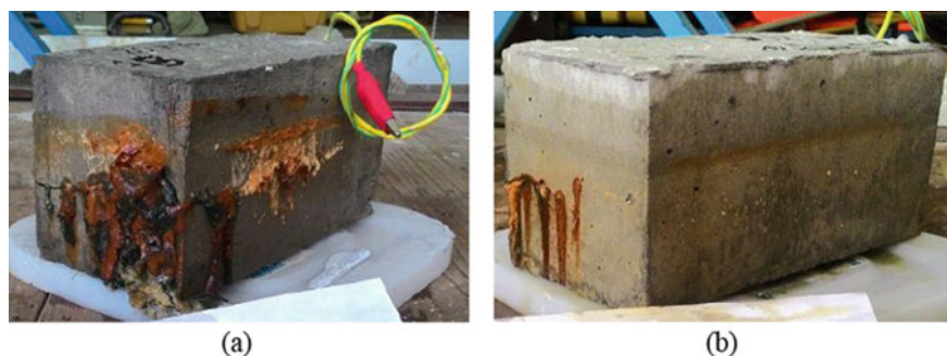
Fig. 1. Concrete without calcium stearate (a), concrete with calcium stearate (b)
