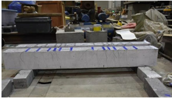
Fig. 6 Electrodes of the smart concrete beam
