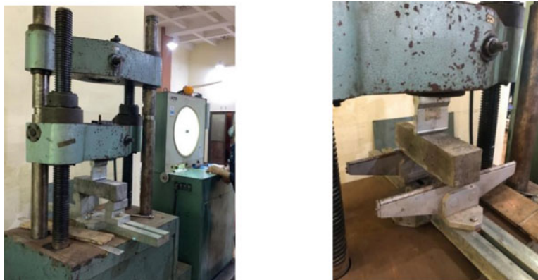
Fig. 3 Modulus of rupture test using Universal Testing Machine
