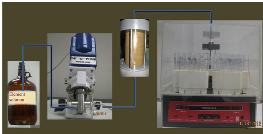
Fig. 12.4 A miscible displacement experimental setup (from left to right: bottle of trace element solution, variable speed piston pump, acrylic soil column, and fraction collector; photos were taken by Elbana, T)
