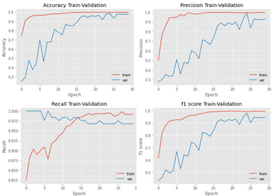
Fig. 2 CNN accuracy, precision, recall, and F1 score in train and validation sets
