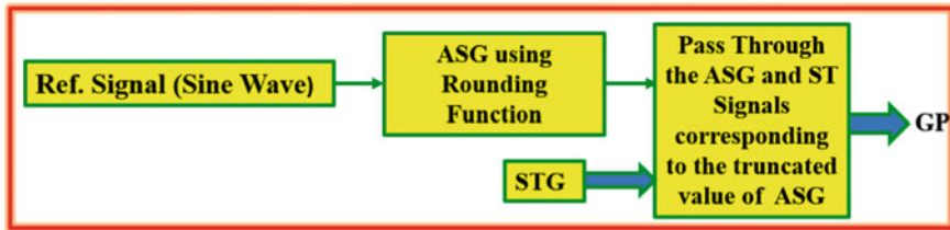
Fig. 2 Unified rounding control scheme-URCS/ULSFCS
