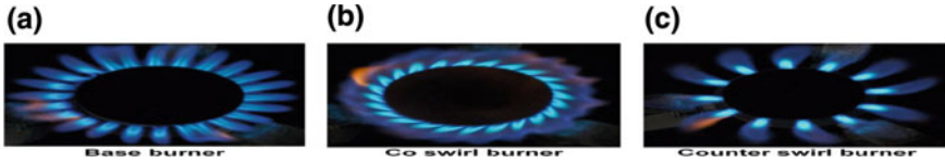
Fig. 5 Flame shape, a no swirl burner ( \theta = 0^\circ ), b co-swirl burner ( \theta = 30^\circ ), c counter swirl burner ( \theta = 30^\circ ). For interpretation of the references to color in this figure, the reader is referred to the Web version of this article
