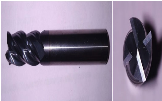
Fig. 3 Coated carbide end mill cutter with 4 flutes
