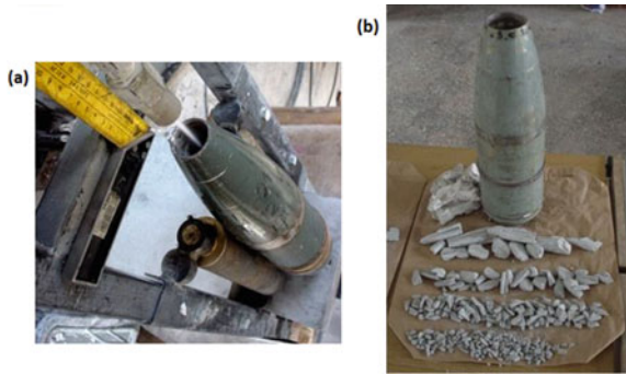
Fig. 2 Waterjet comminution of explosives [15]
