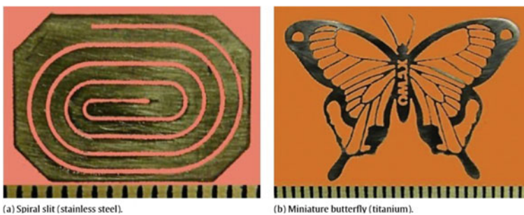
Fig. 4 Micro machined. a Spiral slit (stainless steel). b Miniature butterfly (titanium) [30]
