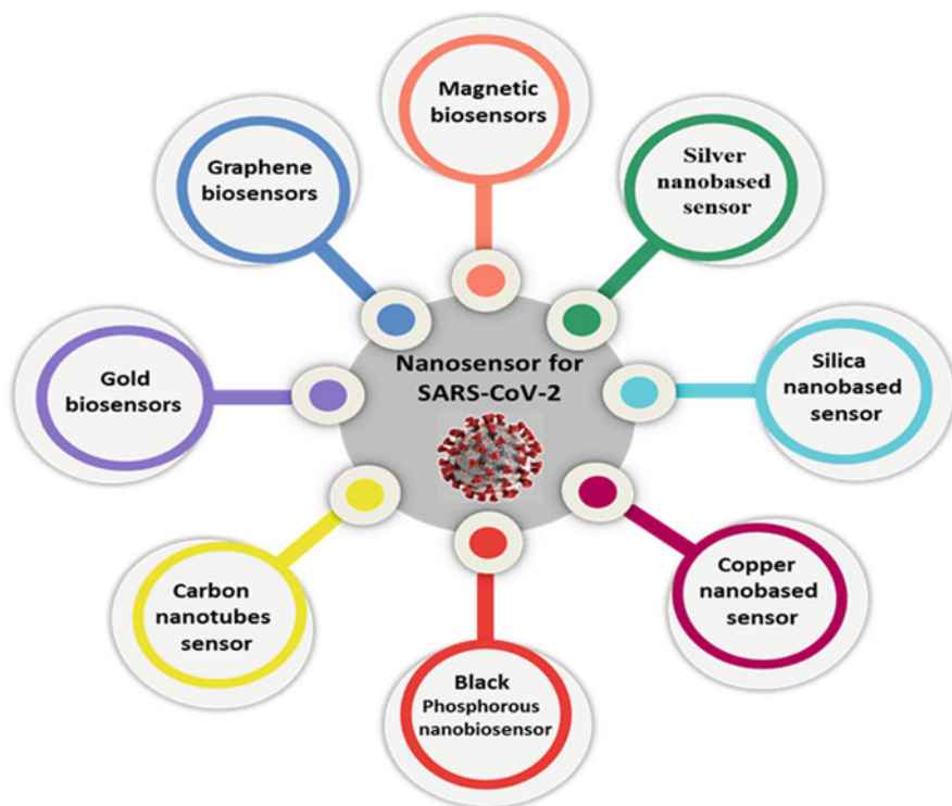
Fig. 23.2 Different nanomaterials that used as biosensor for viral detection
