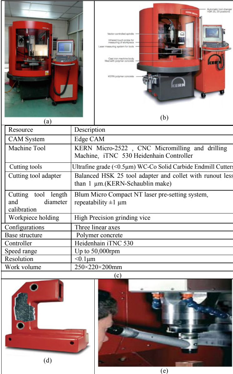
Fig. 1 a Kern Micro-milling, b different systems of micro milling-machine, c features of Kern Micro milling machine, d polymeric concrete construction, e centering microscope
