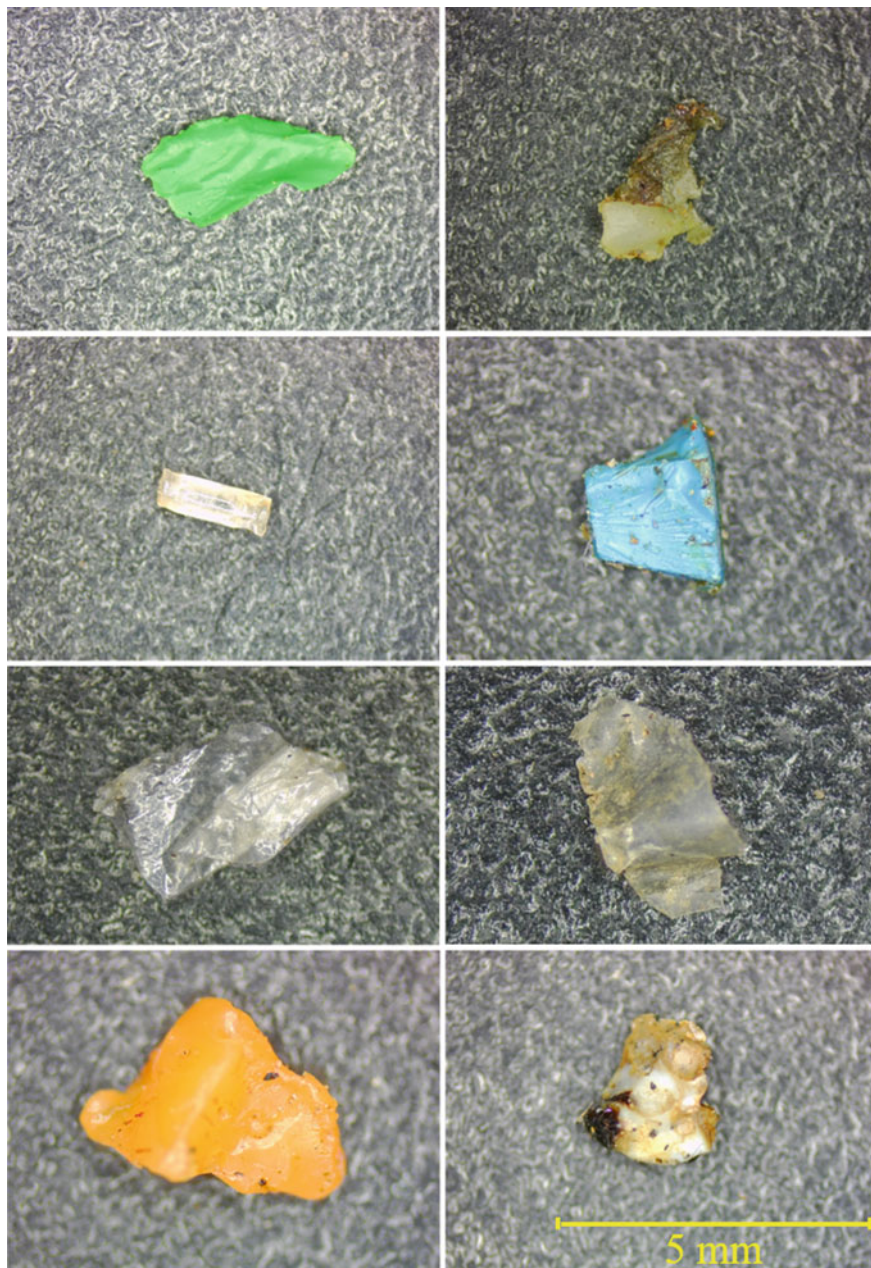
Fig. 9.2 MPs found in the soils of Guiyu, a notable e-waste disassembling zone of China
