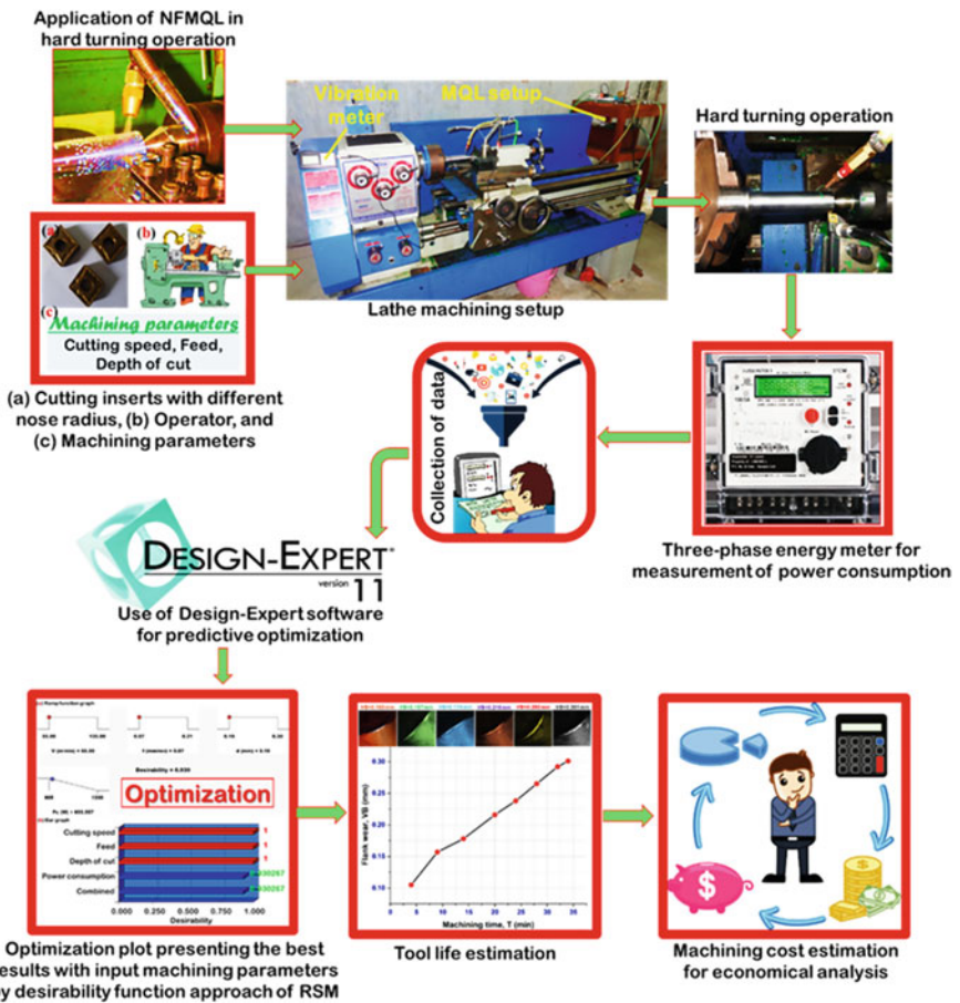
Fig. 1 Schematic of machining setup and procedure for experimental investigation
