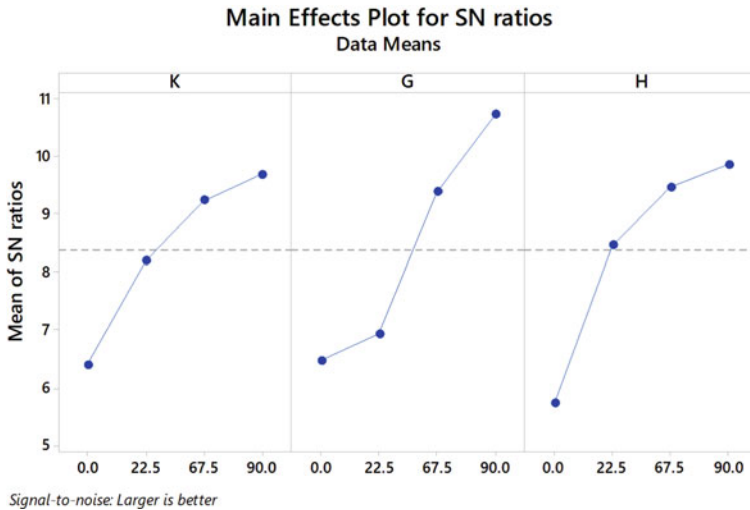
Fig. 3 SN ratio analysis of fiber mixing effects on impact strength
