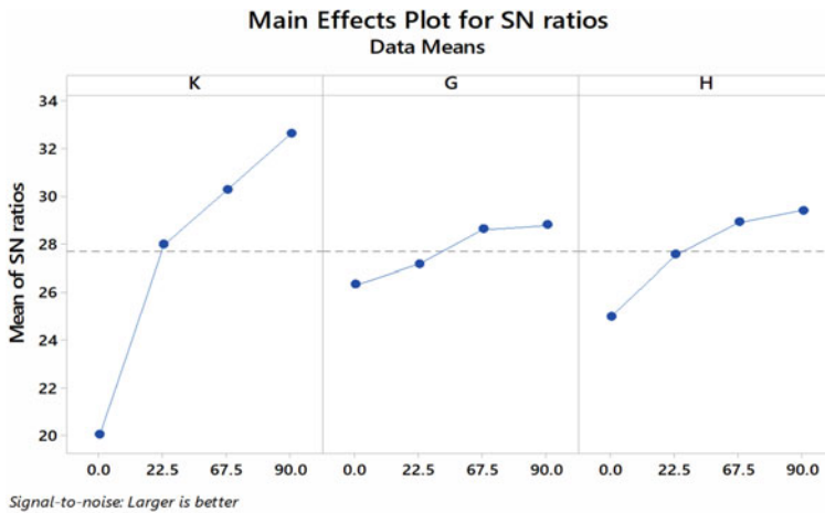
Fig. 1 SN ratio analysis of fiber mixing effects on tensile strength
