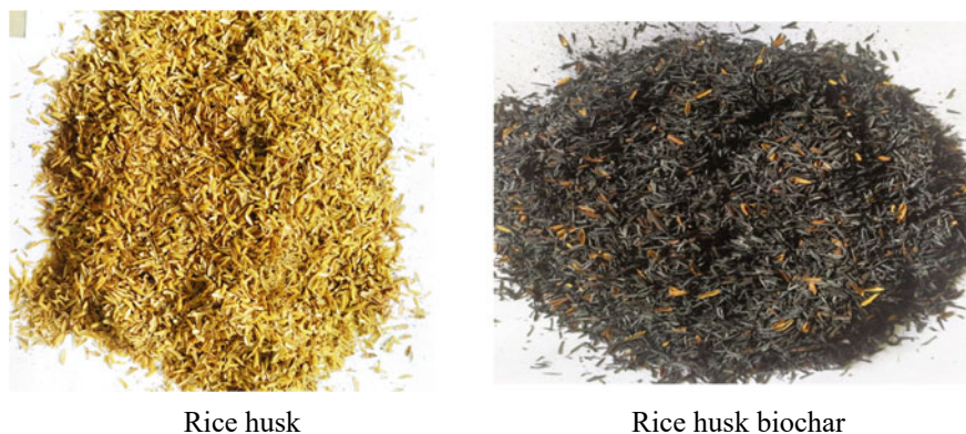
Fig. 1 Photographs of raw rice husk and rice husk biochar
