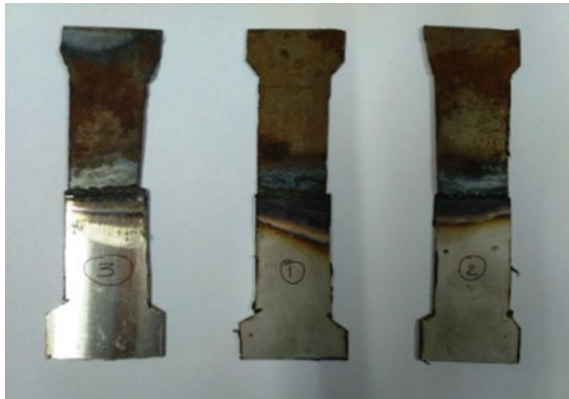
Fig. 1 Tensile specimen of different workpiece material after TIG welding
