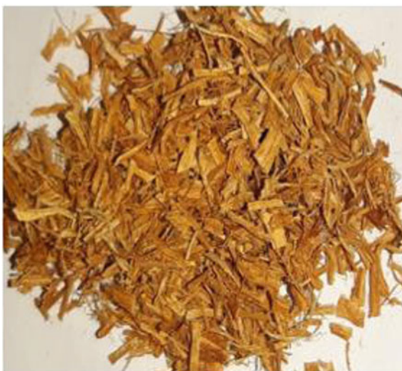
Fig. 2 Chopped BV fibers
