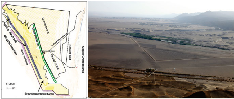
Fig. 10.8 Integrated system combating aeolian disaster map (left, Zhang et al. 2014) and the landscape (right, Wang 2011) on the top of Mogao Grottoes in Dunhuang
