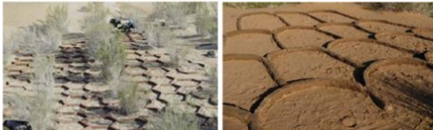
Fig. 8.9 Clay-based sand-fixing composite material sand barriers (Photos courtesy of Ziqiang Lei)
