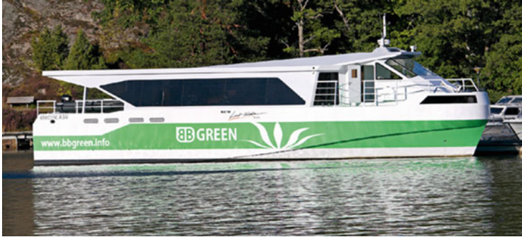
Fig. 5 The 25-ton ship, named BB Green, a first all-electric Air Supported Vessel (ASV) in Riga, Latvia using Leclanché Battery Technology [4]
