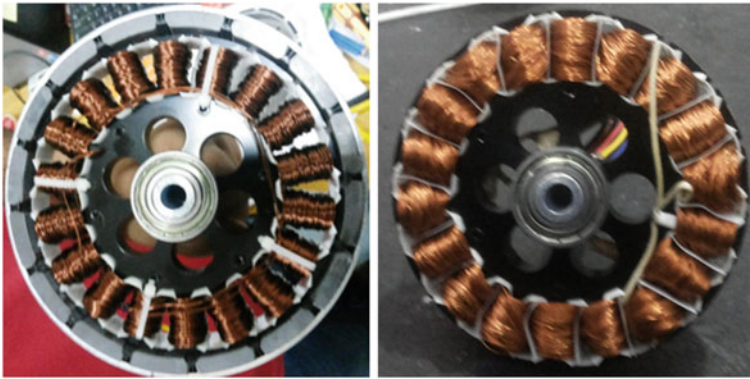
Fig. 5 PMBLDCM based fan winding structures of a available ceiling fan, and b proposed drive
