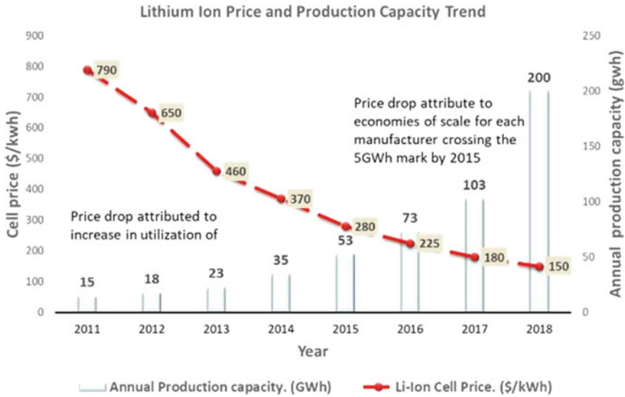
Fig. 2 Battery price and manufacturing capacity trend
