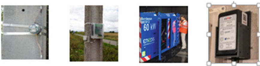
Fig. 4 lightning arrester sensor, fault detector, smart genset, and flood detector
