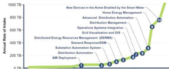
Fig. 6 Pattern of Big data volume in electric utilities
