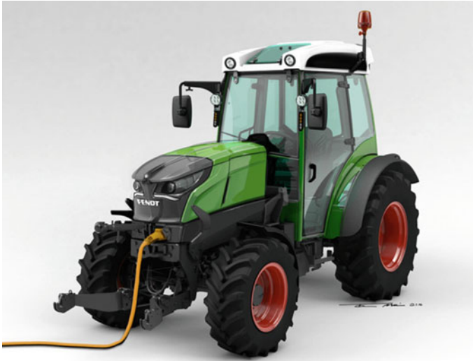
Fig. 7 The Fendt e100 Vario: The battery-powered compact tractor [6]
