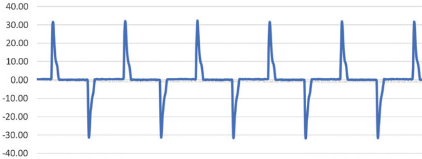
Fig. 7 15 Amp AC charging station input current
