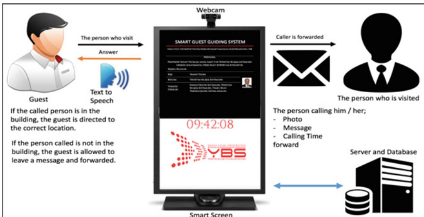
Fig. 2.4 Smart guest guiding system basic structure
