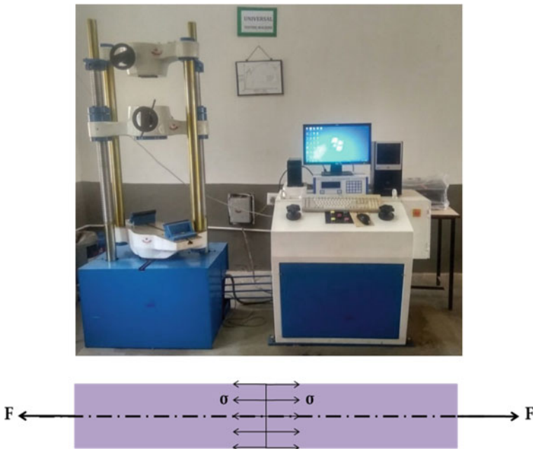
Fig. 2 Tensile test machine and its stress distribution
