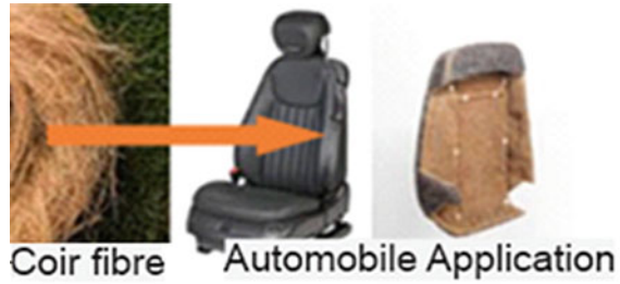
Fig. 3 Application of coir fibre in automobile
