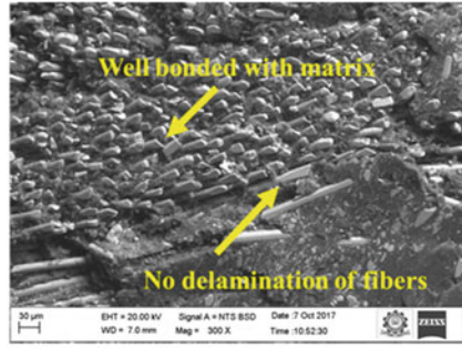
b) Worn surface of Banana composites, wear conditions: load 10N, sliding speed 750 Rpm, 0.5 Wt. % MWCNT
