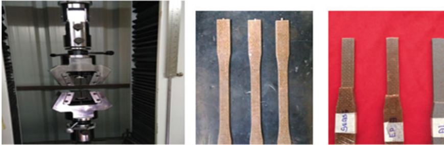
Fig. 6 UTM and specimens before and after tensile test
