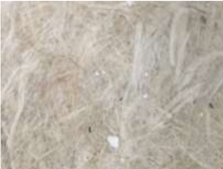
Fig. 3 Prepared composites [15% fiber to 85% epoxy]
