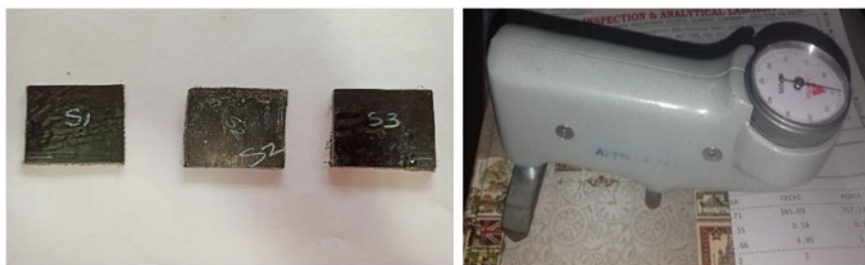
Fig. 9 Hardness test as per ASTM E 2240-05 standard and hardness testing machine
