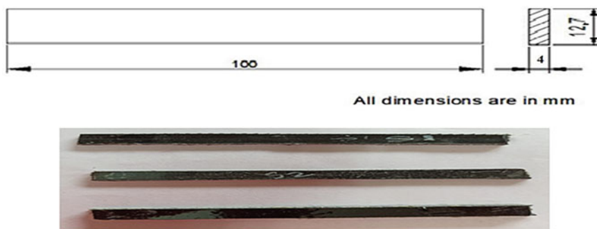
Fig. 5 ASTM D790 standard dimension for flexural test
