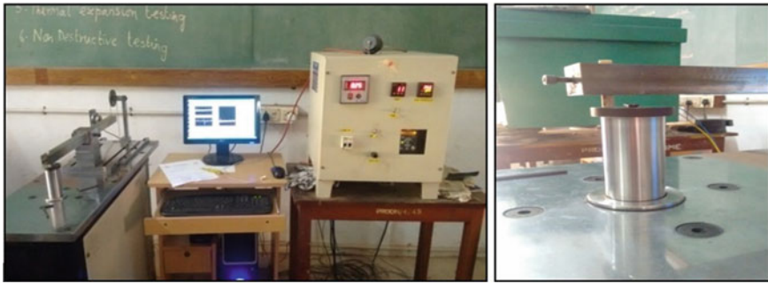
Fig. 2 Pin on disc tribometer experimental set up
