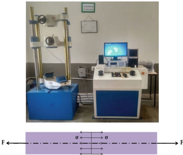
Fig. 2 Tensile test machine and its stress distribution
