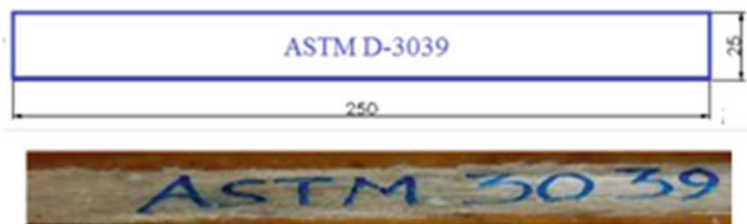
Fig. 4 Test specimens with ASTM D 3039 Standard
