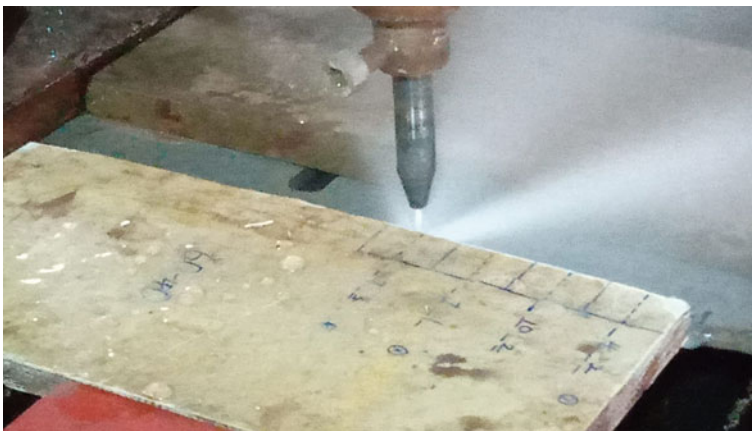
Fig. 1 The cutting zone of AWJ process
