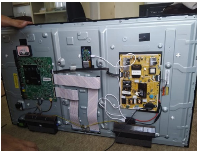
Fig. 3 GPS AND RF interior tagged Samsung LED TV
