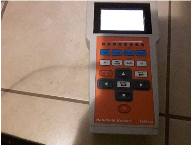
Fig. 6 RF handheld receiver apparatus
