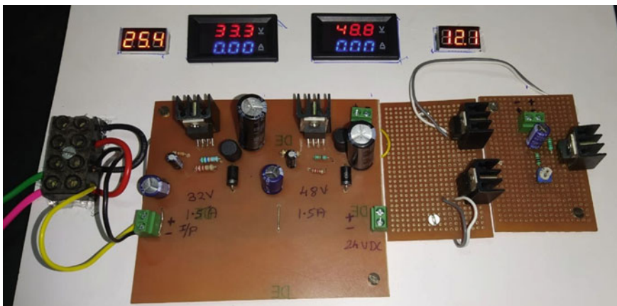
Fig. 7 Experimental setup with display of 12, 24, 32, and 48 V output
