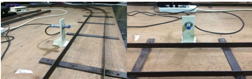
Fig. 14 Sensor for detecting train beside the rail track
