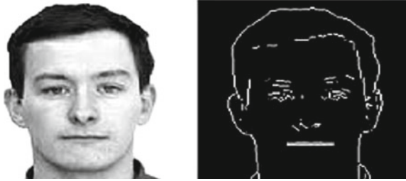
Fig. 5 Sobel edge filter operation of neutral expression of a face sample
