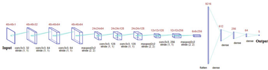
Fig. 4 Proposed DCNN model architecture based on VGG-16 with ELU activation
