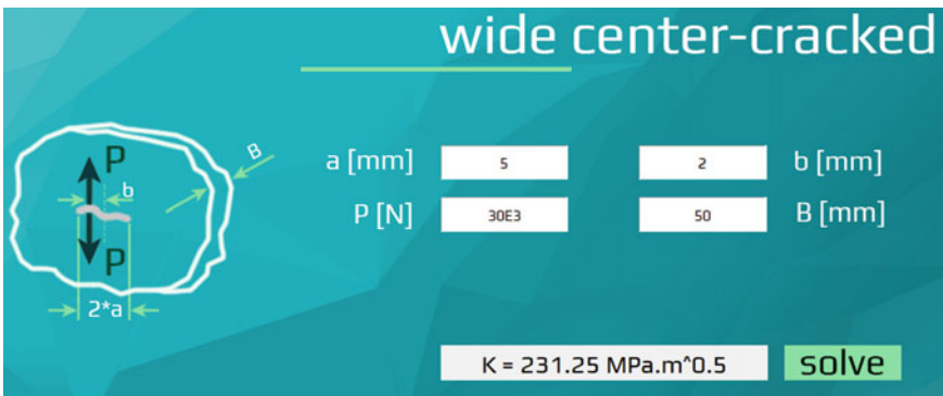
Fig. 6 Wide center-cracked calculation with the aid of the software
