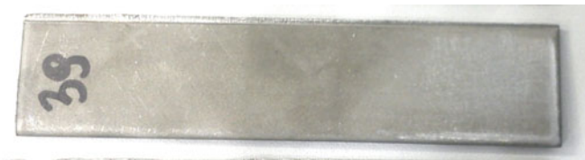
Fig. 2 Example of a sample made of C45 steel with a thickness of 2 mm
