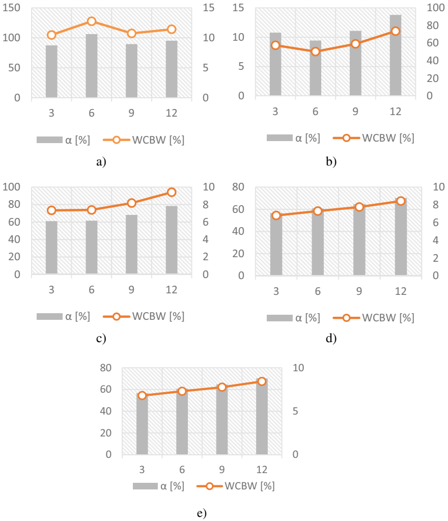
Fig. 2 Development of chemically bounded water and hydration degrees of the mortar samples a CMS-0; b CMS-65; c CMS-75; d CMS-85; and e CMS-95 during the 3, 6, 9, and 12-month bio-corrosion experiment
