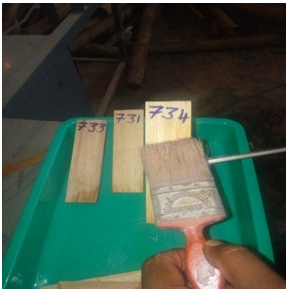
Fig. 16.1 Brush coating of samples
