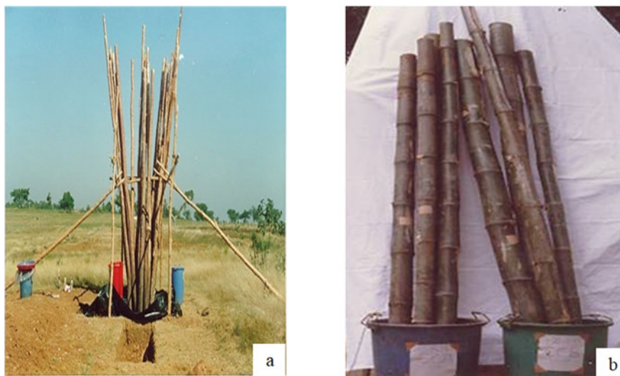
Fig. 16.3 Sap displacement treatment method (a) Eucalyptus poles treated by sap displacement; (b) Bamboo poles treated by sap displacement
