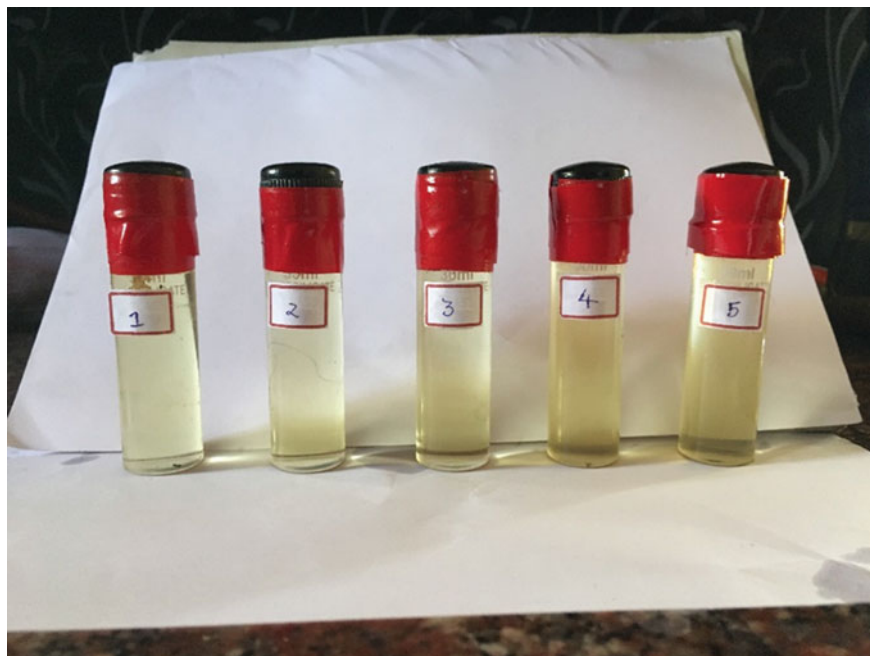
Fig. 8.2 Representative samples of fuel blends kept at 25 °C for a period of 20 days
