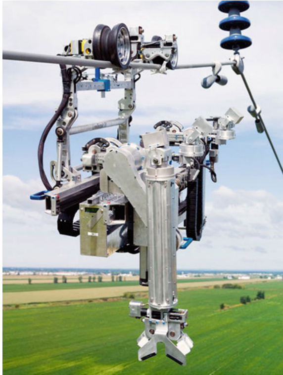
Fig. 7 LineScout climbing on live power lines for routine inspection [9]
