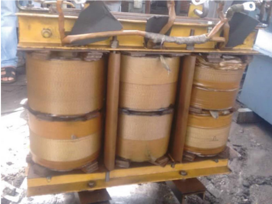
Fig. 3 Internal view of transformer
