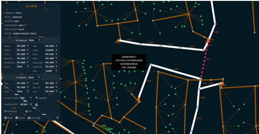
Fig. 3 Vector view of electrical network
