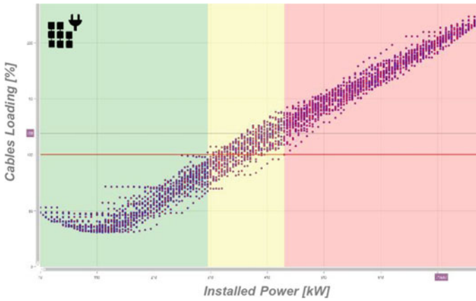
Fig. 4 Result of the module hosting capacity: maximum loading depending on the additional charging power [1]
