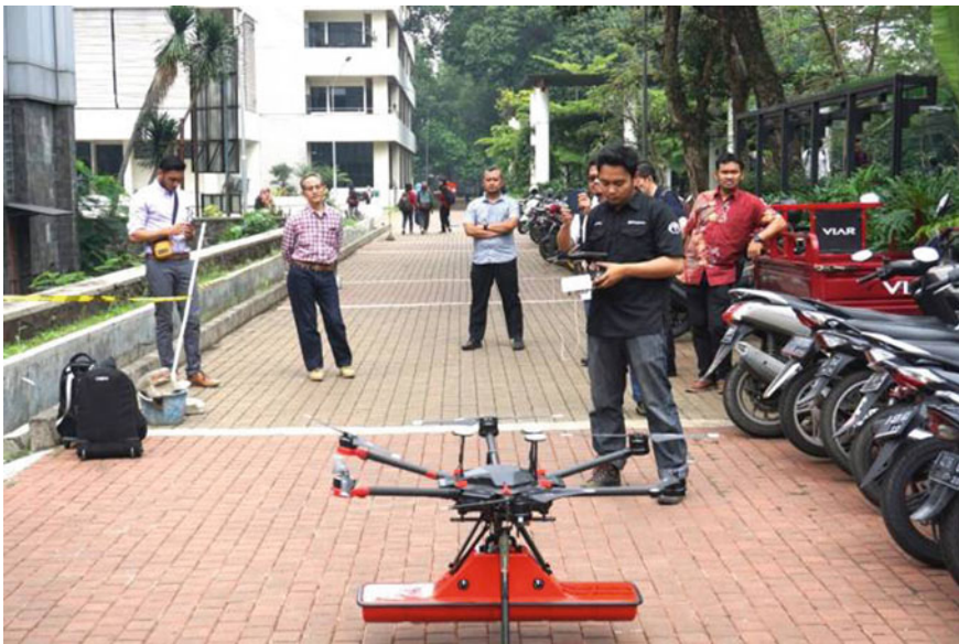
Fig. 3 Pilot project—drone equipped with GPR (ground penetrating radar) system [3, 4]
