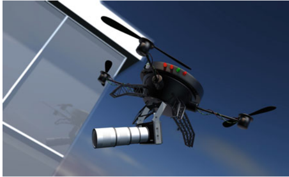
Fig. 2 UAV drone equipped with 4 K HD cameras with infrared capability for surveillance [4, 5]
