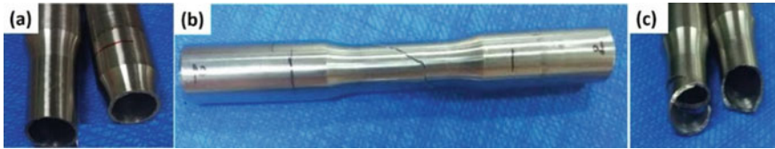
Fig. 12 Different modes of failure for a pure axial, b pure torsion and c combined axial-torsion fatigue tests
