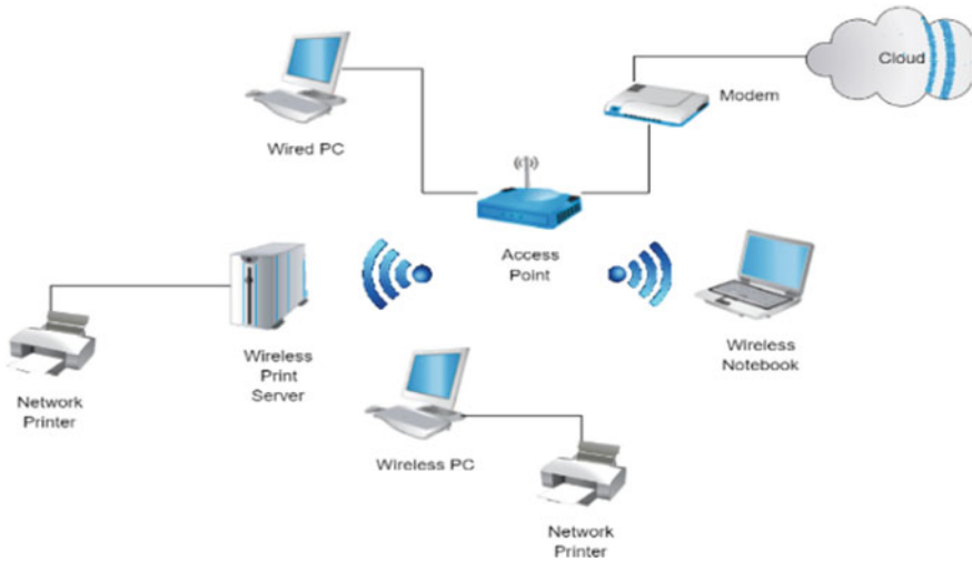
Fig. 1 IoT network architecture inside any small setup like office, school, etc.
