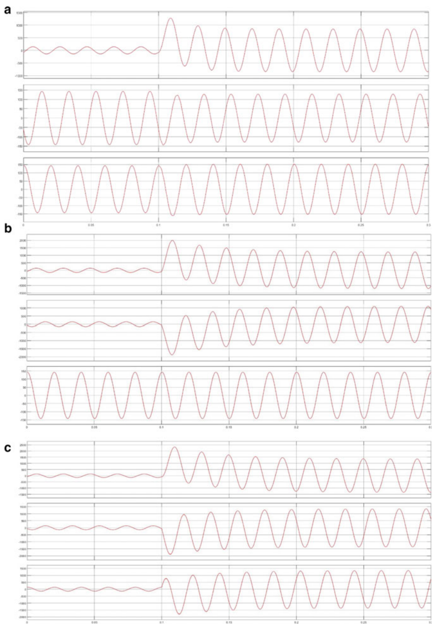
Fig. 5 a System output current waveform of single line to ground fault. b System output current waveform of double line to ground fault. c System output current waveform of three-phase fault.
