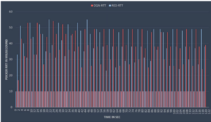
Fig. 5 Plotting packet delay measured by the RTT for each sec in the simulation
