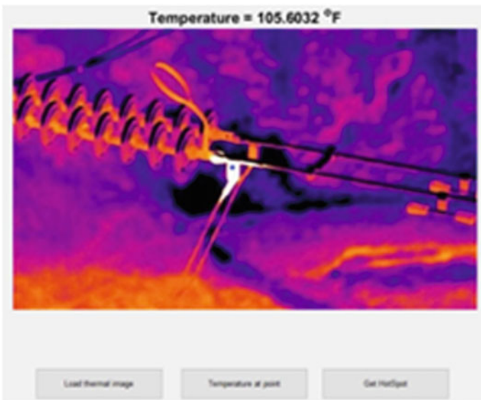
Fig. 5 Temperature of the insulator at the selected point
