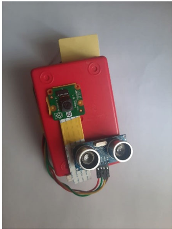
Fig. 2 Experimental setup for crack detection
