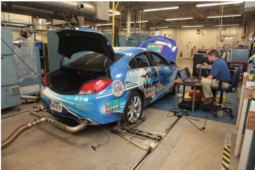
Fig. 6.3 Vehicle installed on a chassis dynamometer at Southwest Research Institute with exhaust emissions sampling lines and emissions sampling unit
