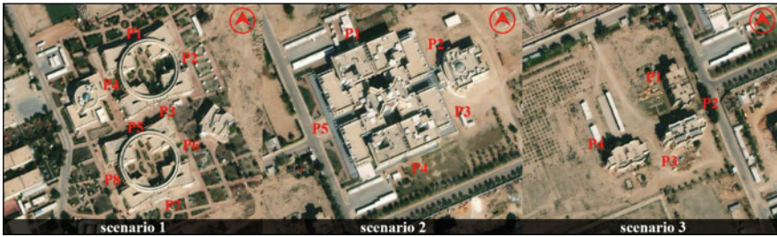
Fig. 2 The measurement positions at 1.75 m from the ground on the university campus
