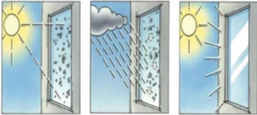
Fig. 6 The basics of how photocatalysis surfaces execute [29]
