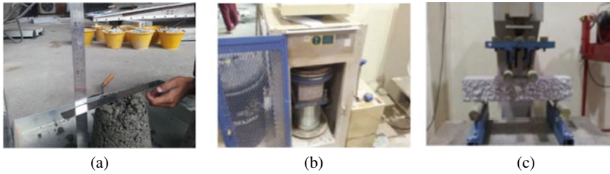
Fig. 1 Laboratory test. a Slump test measurement. b UTM machine for compressive strength and splitting tensile test. c Flexural testing setup using two points loading test
