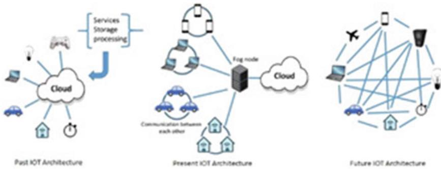
**Fig. 1** Different IoT structures
