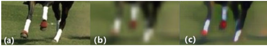
Fig. 8.1 The figure is an example of the SR technique, a is the ground truth, b is the low-resolution image, and c is the recovered high-resolution image
