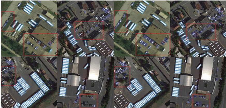
Fig. 8.5 The figure shows visualization results of our method. In the figure, the four pictures on the left are detection results of the S 2 A-Net, and the four pictures on the right are the detection results of our method. Significantly more objects are identified in the red boxes in the four pictures on the right than on the left
