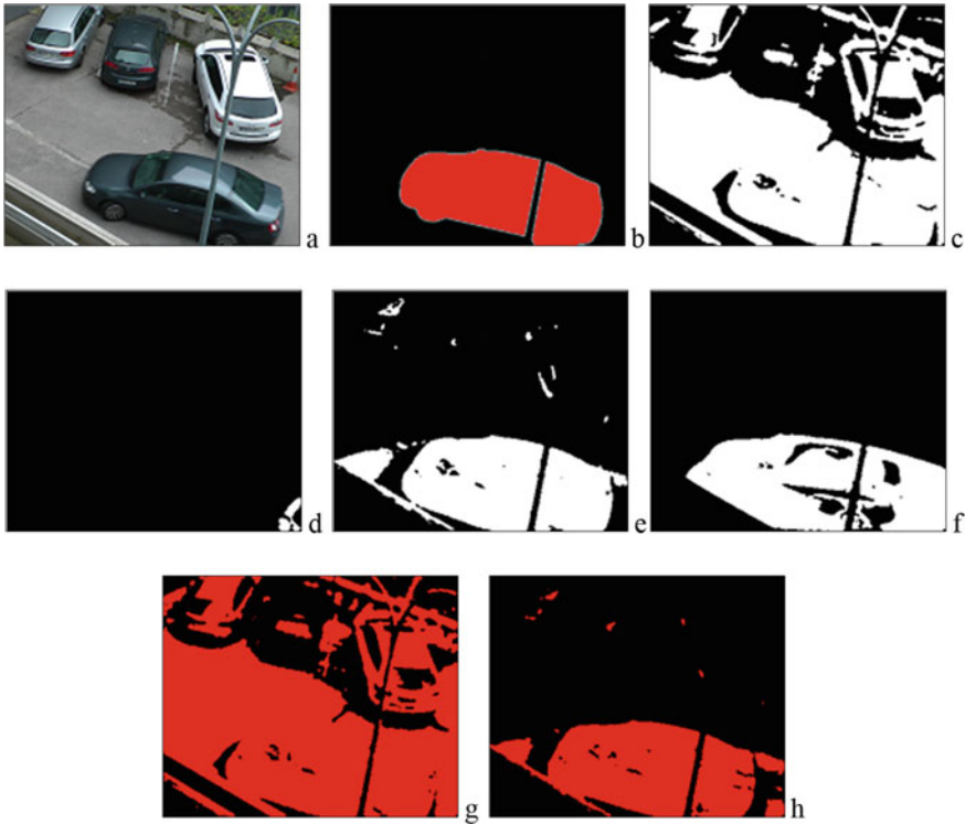
Fig. 2.3 Object detection in a single frame by: a original, b ground truth, c RPCA SSGoDec, d RPCA Lag-SPCP-QN, e NMF ManhNMF, f NMF iNMF, g Fusion OR, h Fusion AND
