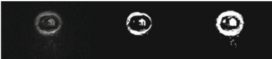
Fig. 6 Binarized images derived by thresholding. Column 1 represents original image, column 2 represents binarized image obtained by the square wave binarization method, and column 3 shows binarized image obtained by Otsu's method [12]
