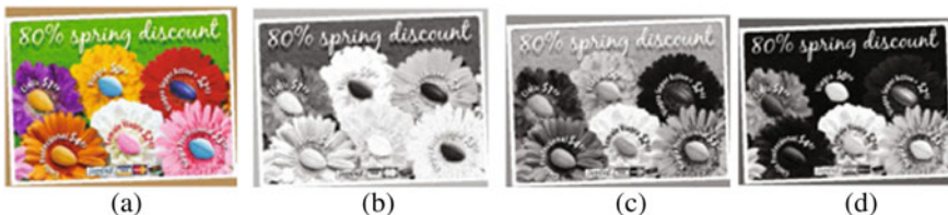
Fig. 8 a Input colored image, b R plane, c G plane, and d B plane
