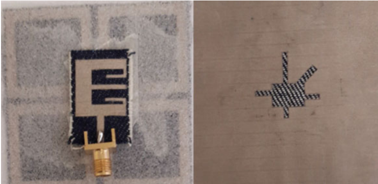
Fig. 11 Fabricated antenna with EBG-DGS designed by Adel Y, Ashyap, 2020, IEEE Access
