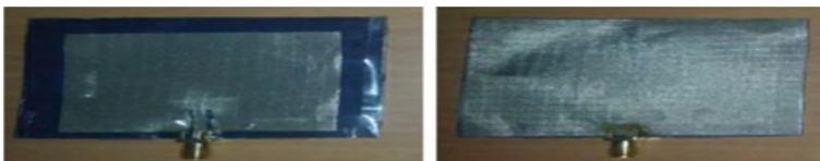
Fig. 1 Front view and back view of nickel copper textile antennas, designed by E. Thangaselvi, 2018, Springer Science + Business Media, LLC, part of Springer Nature
