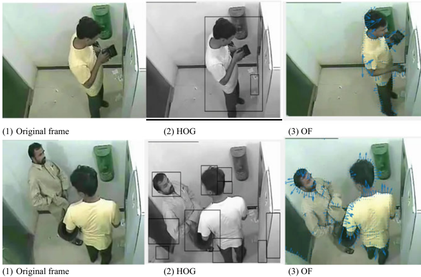
Fig. 5 Abnormal activity detection of frames on ATM surveillance video. Top row: single person: original frames (1), HOG detection (2), and optical flow detection (3). Bottom row: multiple persons: original frames (1), HOG detection (2), and optical flow detection (3)
