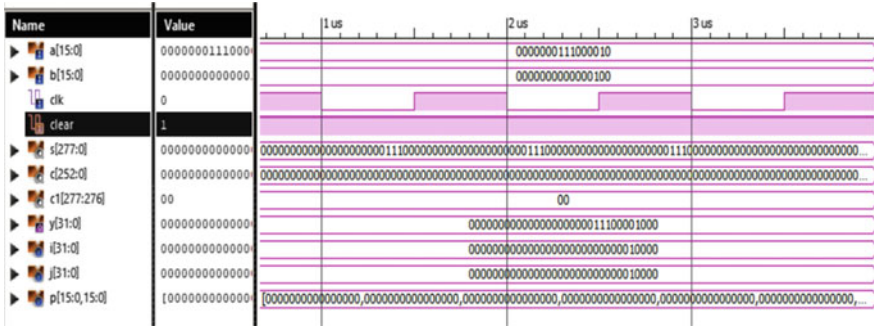
Fig. 8 Simulations results of 16-bit proposed Wallace multiplier using HCA
