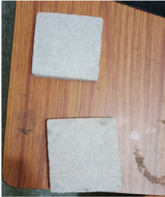
Fig. 5 Sandstone specimens (70 × 70 × 12 mm) for thermal conductivity test
