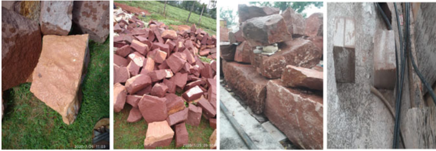
Fig. 2 Sandstone samples collected at the quarry site (Bagalkot, Karnataka) and cut as per standard dimensions
