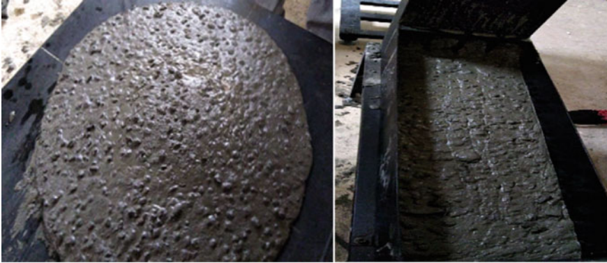
Fig. 1 FA (slump flow + T_{500} ), PA (L-box method) conducted on pozzolanic binary blend SCC
