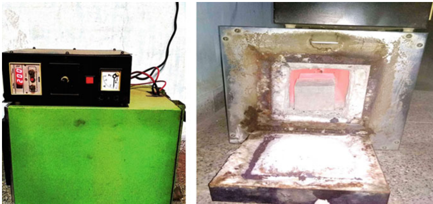
Fig. 1 Automatic electric furnace used for 100–800 °C temperature
