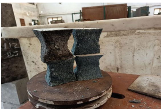
Fig. 2 Failure pattern of mortar cube in compression
