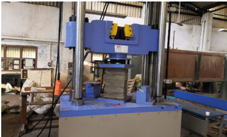
Fig. 5 Compression test on brick prism
