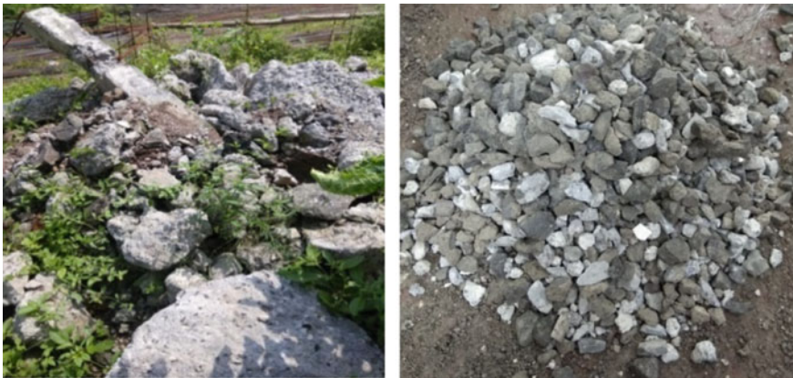
Fig. 1 Recycled coarse aggregates acquired from the demolished structure
