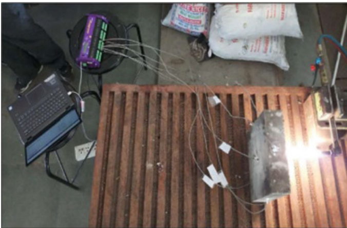
Fig. 2 Specimen under fire exposure
