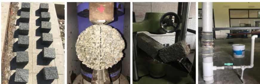
Fig. 1 Specimen for mechanical strength test and testing setup for permeability test and flexural strength test
