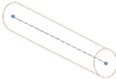
(b) 3-D truss element (T3D2)(for reinforcement)
