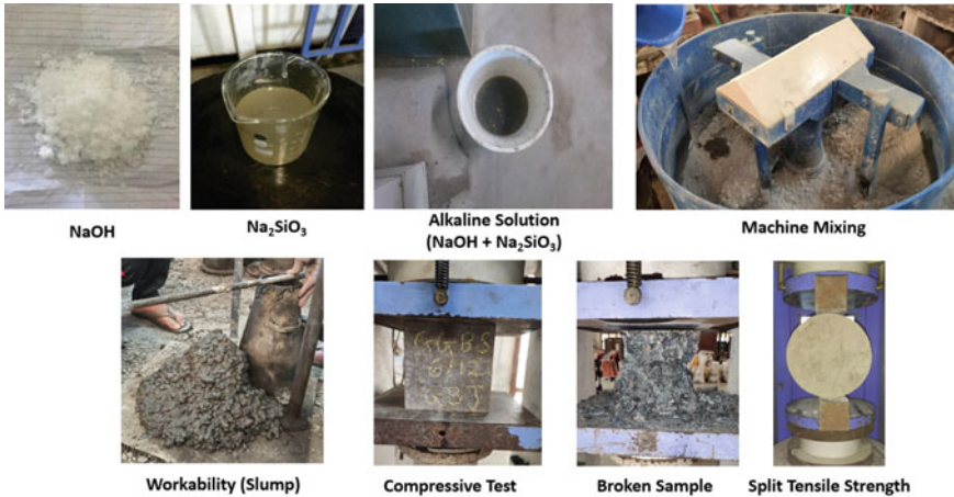
Fig. 2 Casting procedure and testing
