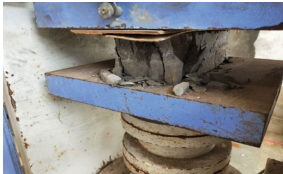
Fig. 3 Brick compression test
