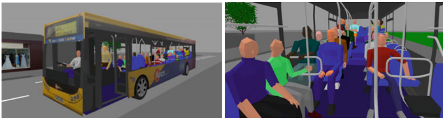
Fig. 10 Bus model reproduced from 3D scanned data for accessibility analysis in DHM
