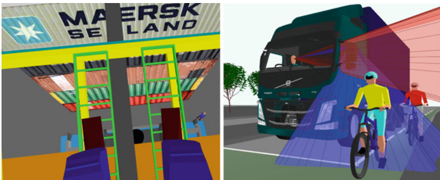
Fig. 5 Visual assessment tools in SAMMIE. Humans view provides a view from the human model's eye (s) (left). Volumetric projections allow the volume of space visible through a window or via a mirror to be visualized (right)
