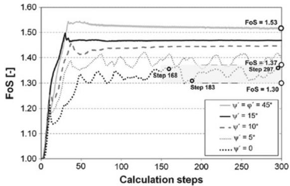
Lin et al. [1] investigated the effect of dilatancy angle on FoS using a 3D finite element model and compared the results with Tschuchnigg et al. [11]. As shown in Fig. 3, using the associated flow rule they observed fluctuations in FoS. They concluded that associated flow rule was not suitable for 3D finite element analysis.
