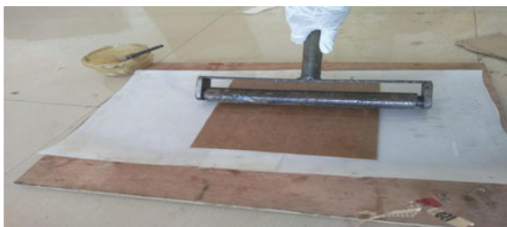
Fig. 2 Preparation of plate specimen
