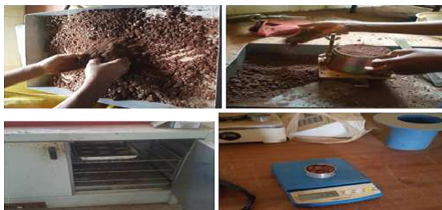
Fig. 6 Standard proctor compaction test for soil–cement mix
