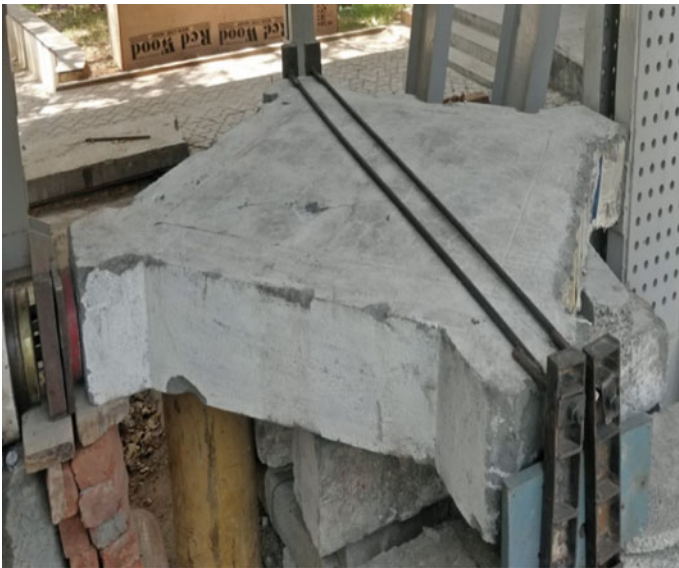
Fig. 8 Test set up for retrofitted specimen RM-S
