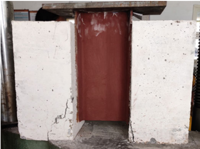
Fig. 7 Concrete crushing failure
