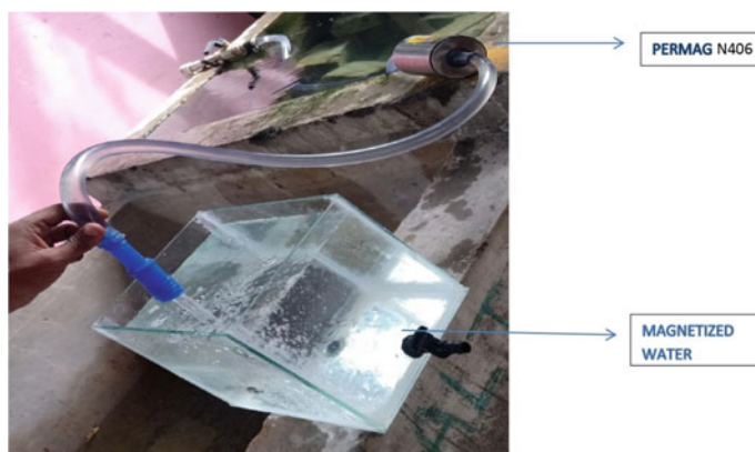
Fig. 1 Magnetic water set-up
