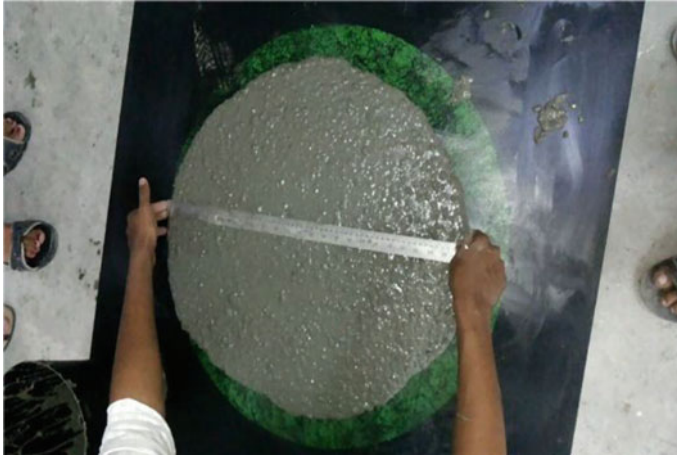
Fig. 1 Flow table test
