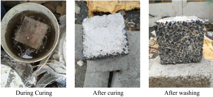
Fig. 5 Process of acid curing
