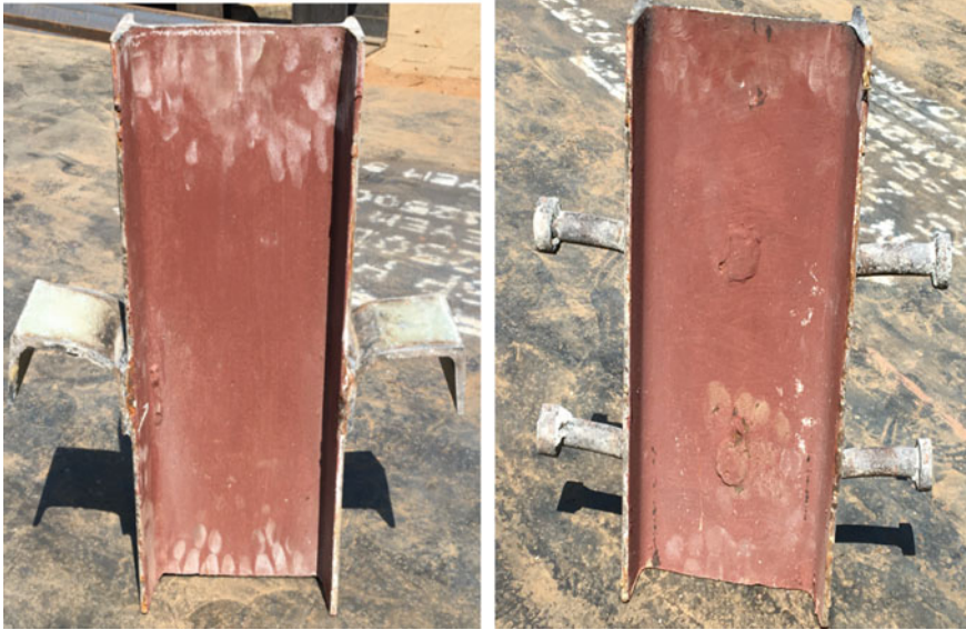
Fig. 10 Buckling of connector
