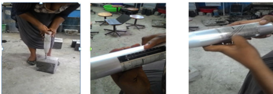
Fig. 6 Rebound hammer testing on concrete
