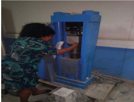
Fig. 4 Compressive strength test setup
