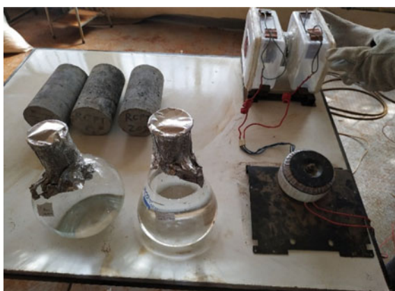
Fig. 7 Concrete discs curing for RCPT
