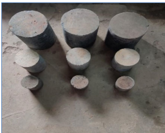
Fig. 6 Top view of cores with varying diameters and heights
