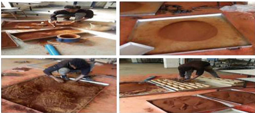
Fig. 4 Preparation of adobe units
