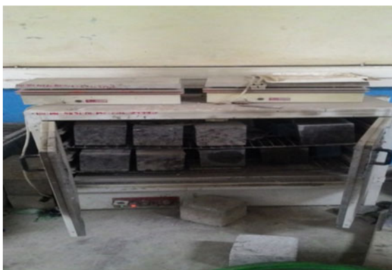
Fig. 10 Concrete cubes in oven for drying
