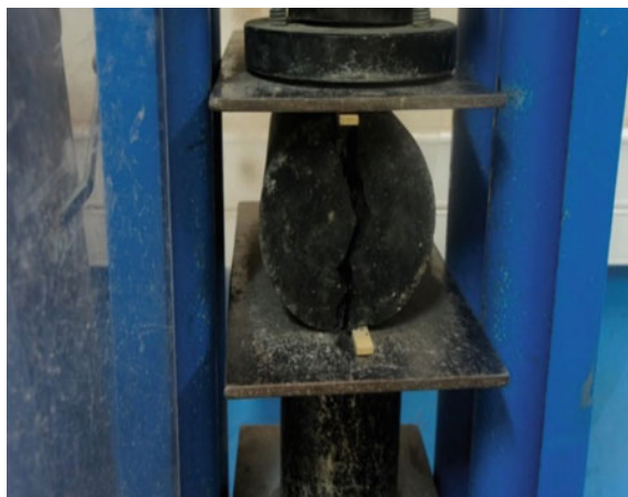
Fig. 5 Tensile strength test setup
