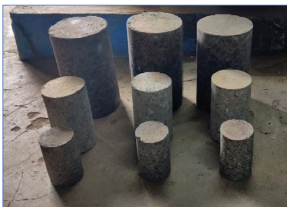
Fig. 5 Front view of cores with varying diameters and heights
