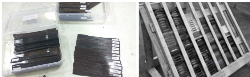
Fig. 3 WPC samples and set up for weathering and aging test
