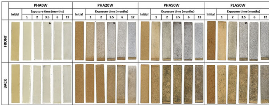
Fig. 1 Visual appearance of PHBV/WF (0, 20 and 50 wt% WF) and PLA/WF (50 wt%) composite samples when exposed to natural weathering. FRONT (top row): the surface facing the sun; BACK (bottom row): the surface in the shade. Figure adapted with permission from (Chan et al. 2019) and modified, Elsevier, copyright 2019
