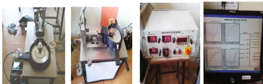
Fig. 2 Wear and friction tester, digital controller box, reading on MAGVIEW-2010
