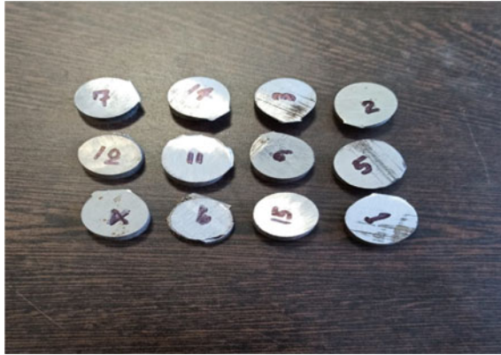
Fig. 6 EDMed removed work surface
