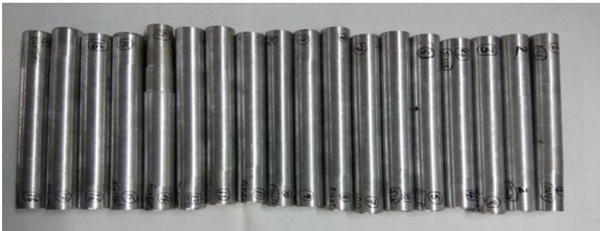
Fig. 1 Specimens of A7075 reinforced with fly ash and SiC
