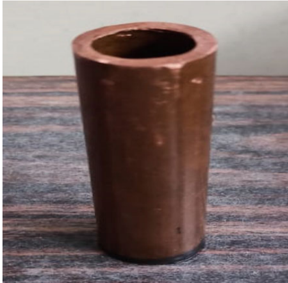
Fig. 3 Hollow shape copper tool
