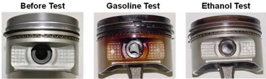
Fig. 2.3 Piston and ring images before and after the test for gasoline- and ethanol-fuelled engine in an end-to-end test of a flex-fuel engine (Santos Filho et al. 2018)
