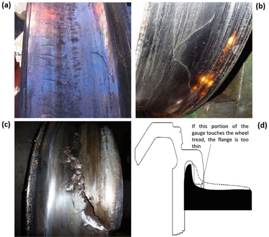
Fig. 5.2 a Rolling contact fatigue wear in rail wheel, b sub-surface fatigue crack, c propagation of sub-surface fatigue crack, and d thin flange gauge (Transport 2021)
