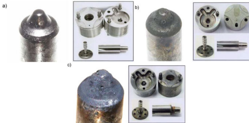
Fig. 3.12 Injector deposit with a RME5 fuel, b RME30 fuel, c RME30 fuel aged for 16 weeks. Adapted with permission from Urzędowska and Stępień (2016) Copyright 2016 Elsevier
