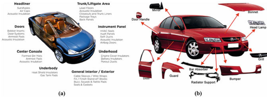
Fig. 10.5 a Interior trims (UFP Technologies 2021) and b Exterior trims of an automobile (Jasonstathamnz 2015).
