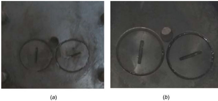
Fig. 3.2 Carbon deposits on the cylinder head from biodiesel and diesel-fueled vehicles after the long-term field test. Adapted with permission from Singh et al. (2019c) Copyright 2019 ASME
