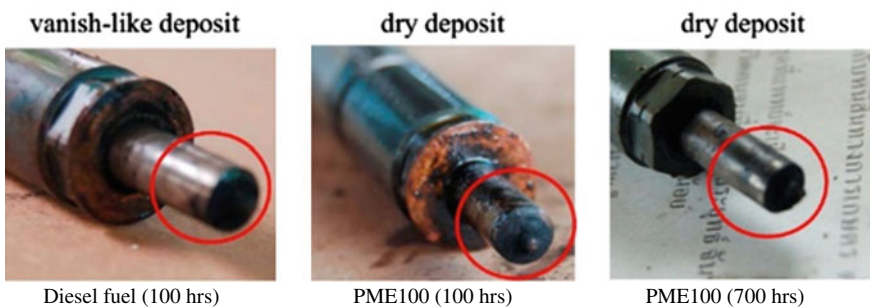
Fig. 3.9 Carbon deposits on fuel injector. Adapted with permission from Suthisripok and Semsamran (2018) Copyright 2018 Elsevier
