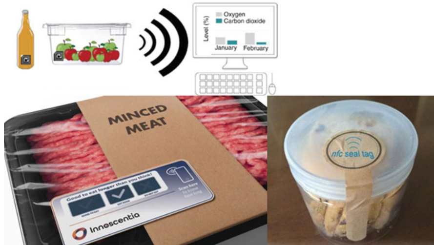
Fig. 9.3 Safety of consumables can be monitored using RFID technology. With sensor integration the safety of the food product can be determined by analyzing the gas content of the package which determines the safety of the product
