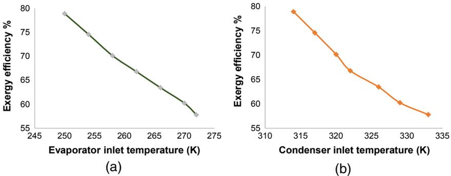
**Fig. 3** Behaviour of exergy efficiency with **a** the evaporator inlet temperature and **b** the condenser inlet temperature
