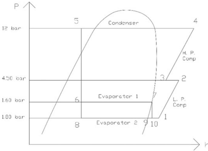
**Fig. 2** Representation of system on P-h chart
