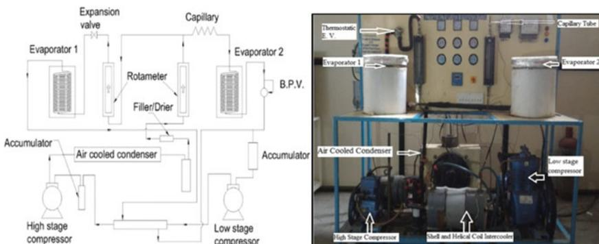
Fig. 1 Diagrammatic demonstration and real picture of the experimental setup
