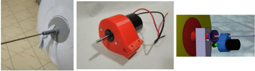
Fig. 6 3D printed pipe and the stainless-steel shaft mounted on the balloon, generator in its mount, CAD model for the translation mechanism
