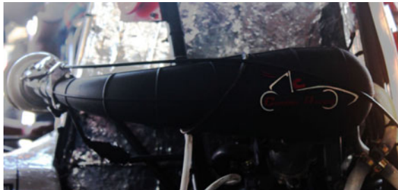
Fig. 18 Real Intake system
