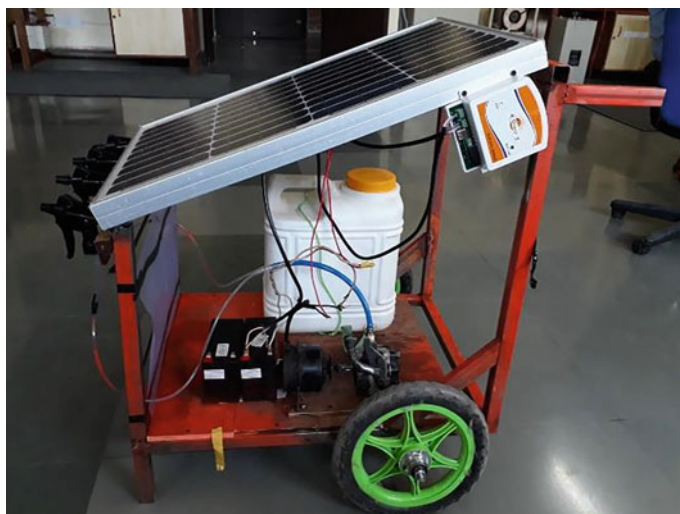
Fig. 4 Final fabricated model for the solar powered spray pump system
