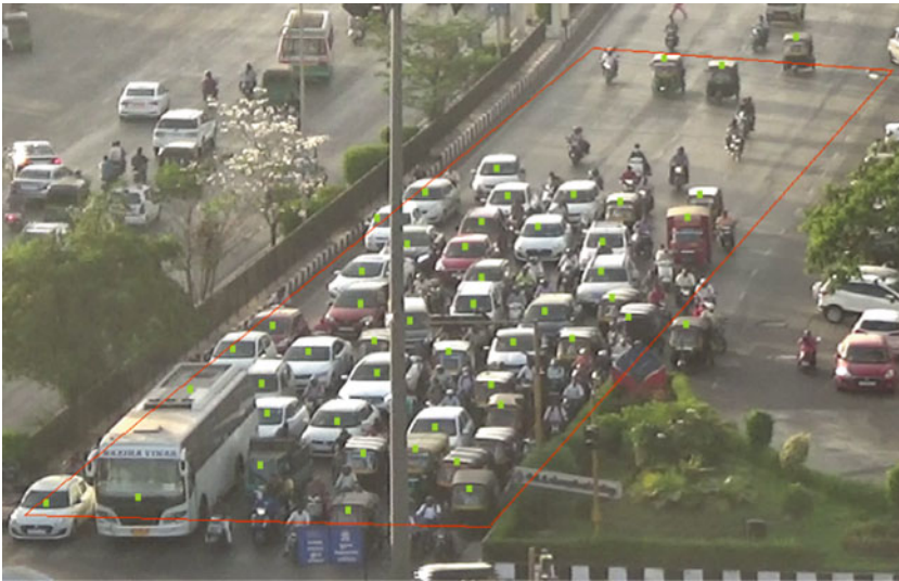
Fig. 3 Screenshot during vehicular trajectory data extraction using TDE
