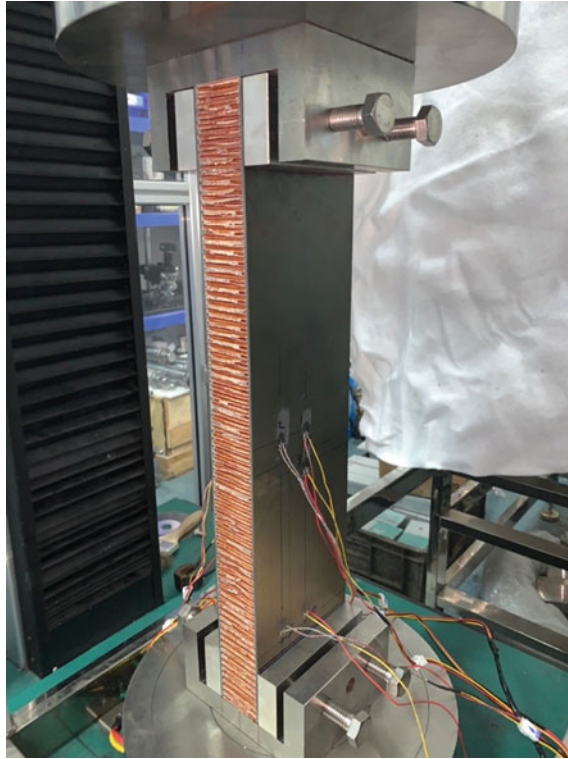
Fig. 7 Edgewise compression test for honeycomb sandwich panel
