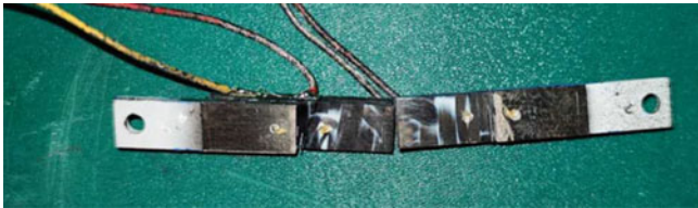
Fig. 9 Interlaminar shear specimen failure
