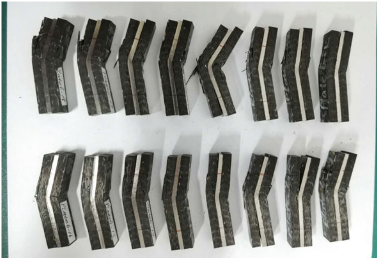
Fig. 20 Failure of short-beam shear specimen
