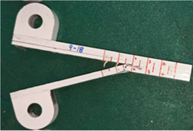
Fig. 31 Interlaminar fracture sample Mode B
