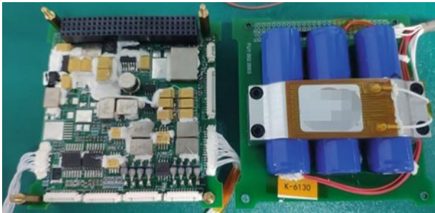
Fig. 5 The electrical power system
