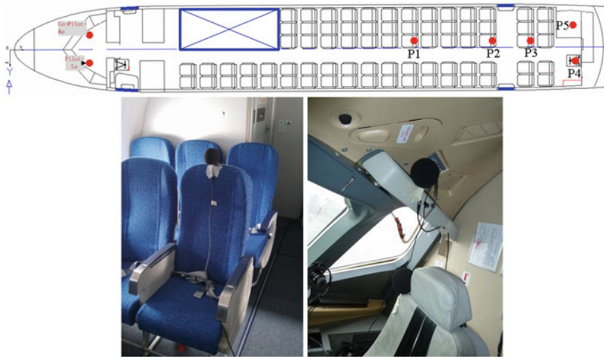
Fig. 11 Microphone site of acoustics experiment on airplane
