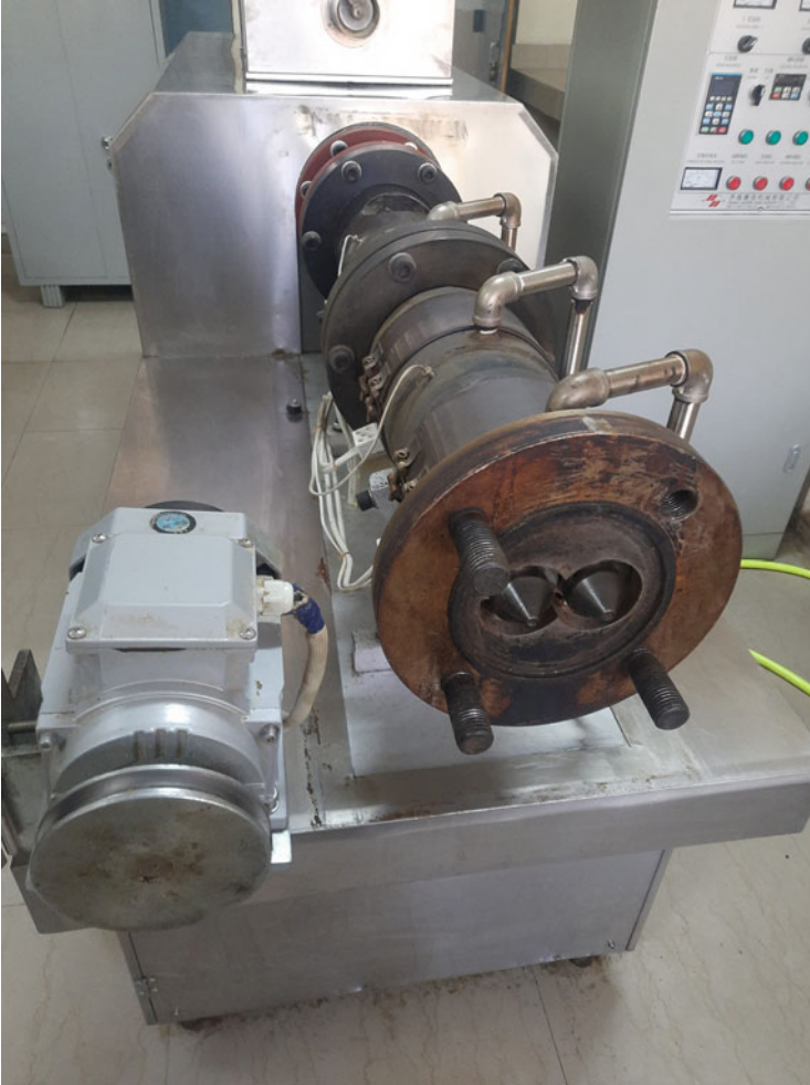
Fig. 14.2 Double screw extruder (Source: Product Development Laboratory, Department of Livestock Products Technology, Guru Angad Dev Veterinary and Animal Sciences University, Ludhiana, Punjab, India)
