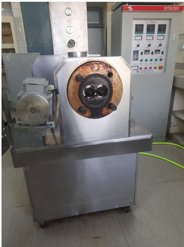
Fig. 14.1 Double screw extruder (Source: Product Development Laboratory, Department of Livestock Products Technology, Guru Angad Dev Veterinary and Animal Sciences University, Ludhiana, Punjab, India)
