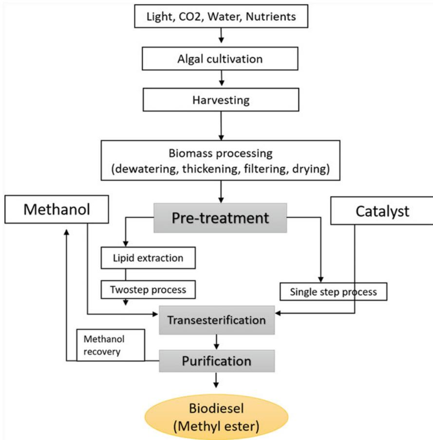
**Fig. 13.3** Production of biodiesel through algal cultivation
