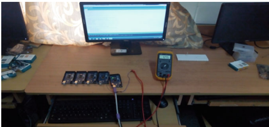
Fig. 11 Case study setup of analysis of random mismatch variations in microcontrollers
