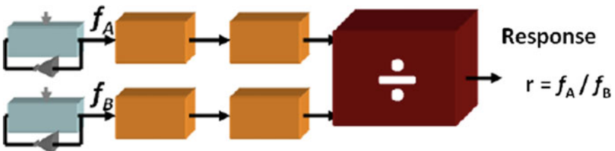
Fig. 7 Ring oscillator with division compensation approach
