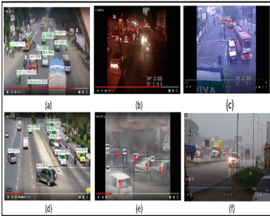
Fig. 3 Multi-vehicle detection, tracking and classification in distinct visual conditions (a day b night c early morning d sunny e rainy f foggy) using SSD algorithm (best viewed in color)
