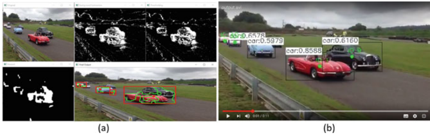
Fig. 2 Comparison of multi-vehicle detection and tracking using a state of art methodology b single shot detector (best viewed in color)
