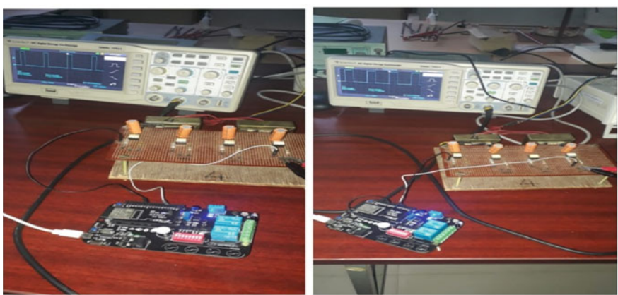
Fig. 10 Gate pulse of variable duty generated from SPELEC board
